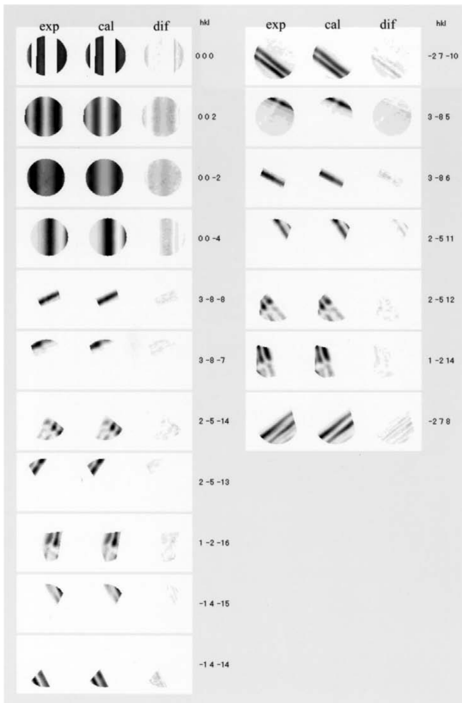
Fig. 9. Final result of the fitting using the data of Fig. 8 taken with the 00 \bar{2} Bragg position.
